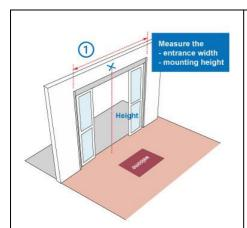
**Step 1**: Determine the mounting location (ideal height: 2.8m – 3.5m), calculate the total counter required using <u>FootfallCam Calculator</u>
