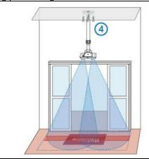
Step 3: Mount the drop pole onto the ceiling.
