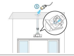
**Step 4**: Connect the Cat5 cable through the tubes of the drop pole.
