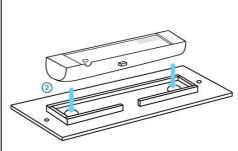
**Step 2**: Attach the counter to the bracket.
