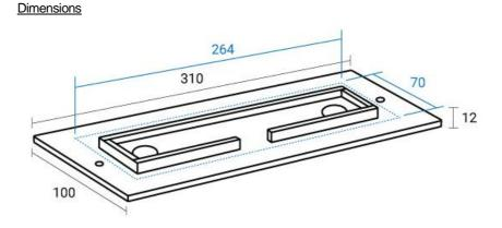
FootfallCam Flush Mounting Plate Kit FC-FMP04
