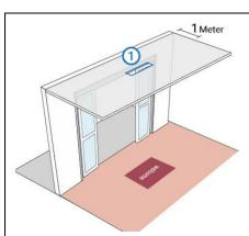
**Step 1**: Determine the mounting location (ideal height: 2.8m – 3.5m), cut the hole of camera space for installing the mounting plate (**264mm x 70 mm**)
